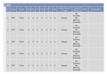
**3.** Check [Enable Image Buffer/Transfer], and select [Timer] for the trigger, and click [Next>].
